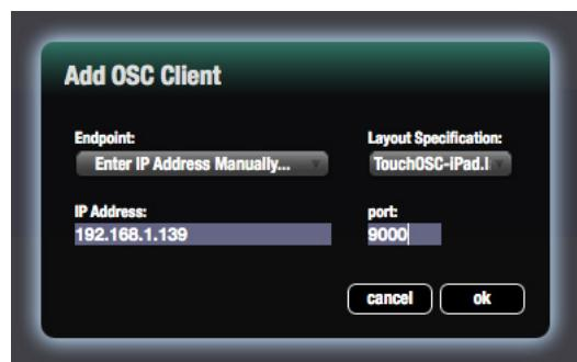
Figure 6: Entering the IP address manually for devices that don't use Bonjour.
